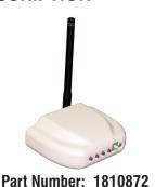
The addressable Universal RTS Interface II (URTSI II) can be used to communicate between home automation or other third party systems and SOMFY's RTS Motors and controls. It is capable of individual or group control, and can be operated via infrared remote, RS232 and RS485 serial communication. Once an input is activated, an RTS radio command is sent to the automated window treatment.
